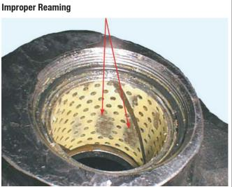
**General Description:** Damaged bushing material, areas of bushing material bunched up or missing, or gouges in bushing
