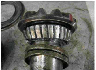
**Helical Thrust Washer - Water Damage**
