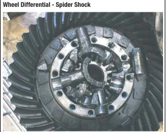
Wheel Differential - Side Pinion Shock
