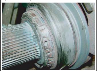
**Output Side Gear Bearing - Low Lube**
