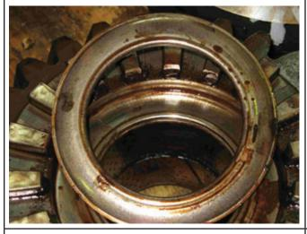
Helical Side Gear Bushing - Water Damage
