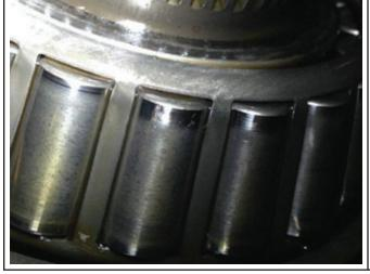
Differential Cage Bearing Cup - Overload - Excessive Wear
