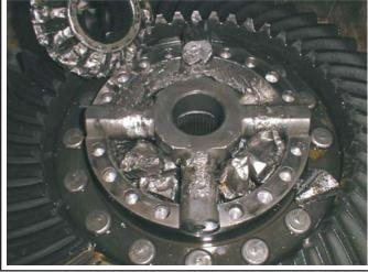
Wheel Differential Spider Arm - Galling, Welded
