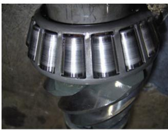
**Input Bearing - Denting - Contamination**
