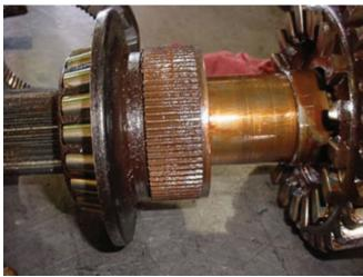
**Input Bearing Cone - Water Damage**
