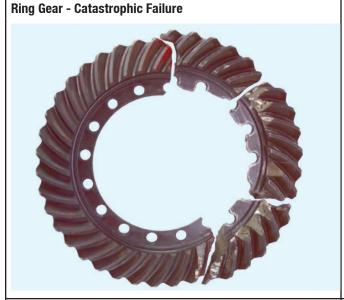
Ring Gear - Coast Side Shock Failure
