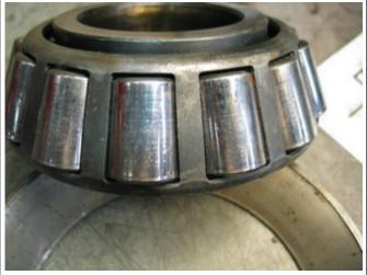
**Bearing - Lack of Lubrication**
