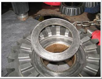
**Power Divider Spinout - Stub End Galling**
