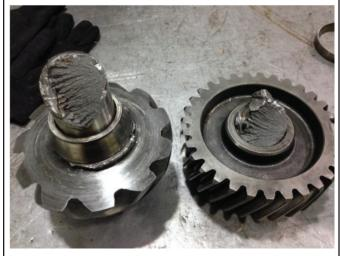
**Drive Pinion - Tooth Shock Load Failure**
