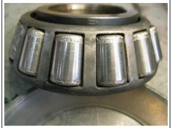
**Pinion Bearing - Hard Contamination**
