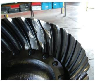
**Ring Gear - Coast Side Shock Failure**
