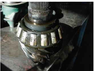
**Bearing - Excessive Bearing Preload - Heat**
