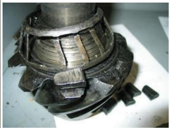
**Bearing Cone - Spalling - Water Damage**
