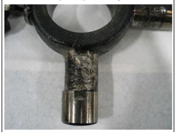
Wheel Differential Side Pinion - Spinout Galling
