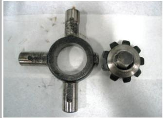
**General Description:** Spinout is excessive wheel spinning that produces damaging heat. High heat breaks down lube film,
