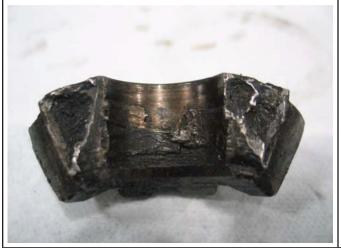
Thrust Washer to Input Shaft - Galling
