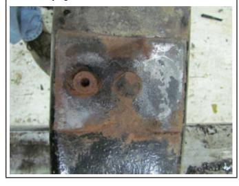
General Description: Sufficient clamp load at the spring pad area is important to keep the joint tight. Loose clamping or
